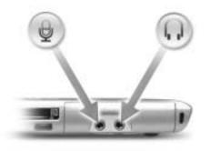
Attach a microphone to the  $\Theta$  connector.
